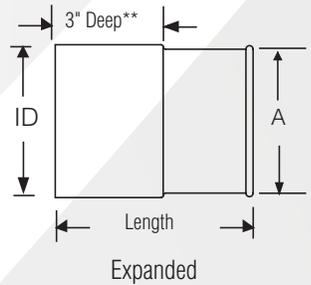
**Adapters can only be expanded up to .3" above the nominal diameter size (A dimension). Expansions larger than .3" must be ordered as a reducer.**
