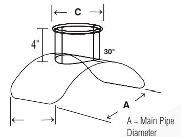
Saddle length and width = 2" all directions from Branch Tube C.
