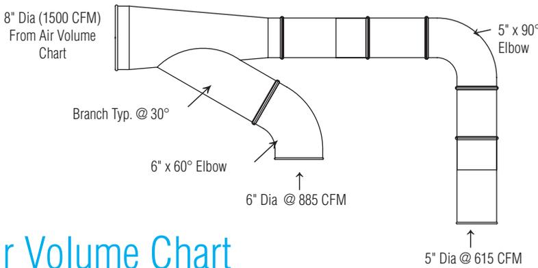
The 5" pipe carries 615 CFM at 4500 FPM, (See chart). The 6" pipe will need 885 CFM at the same velocity (See chart). Added together you have a total of (615 + 885) 1500 CFM coming together.
