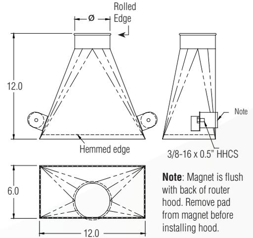
**Note:** Magnet is flush with back of router hood. Remove pad from magnet before installing hood.
