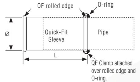
The Quick-Fit Sleeve provides an easy way to adjust for straight duct sections shorter than 5'
