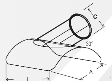
Saddle length and width = 3" all directions from Branch Tube C. A = Main Pipe Diameter
