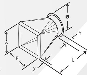
\*NOTE: Minimum L = .75 (B). If less, square to square transition will be provided. 7" minimum L allowable for Sq to Rd and 4" L minimum allowable for Sq to Sq.
