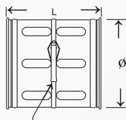
To adjust, loosen QF Clamp and turn outer sleeve to get proper airflow. Re-clamp when finished.
